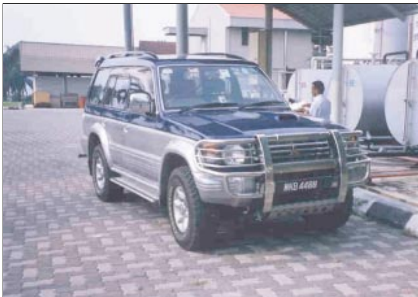
Figure 4. One of the MPOB Pajero participating in the exhaustive field trial using B5 processed liquid palm oil/petroleum diesel blend.
