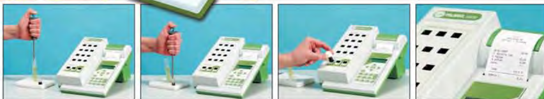
Each test is run by dispensing a preset minimum amount of sample directly into the cuvettes containing the buffer. The special reagents developed for the system produce a colorimetric reaction. The test result is printed directly, after the photometric measurement has been processed, in an appropriate unit of measurement.
