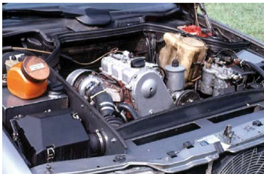
Figure 1. Crude palm oil used directly to run a car fitted with an Elsbett engines.
