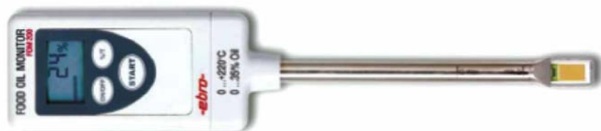
Figure 2.6 The FOM 200 Instrument for Dielectric Constant in Hot Oil
