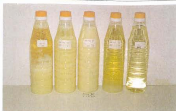
Figure 4(b). Cold stability of blends of single fractionated palm olein with sunflower seed oil after three months at 15°C. The blends are the same as in Figure 4(a).
