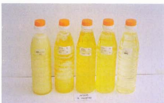
Figure 5(a). Cold stability of blends of double-fractionated-palm olein (IV60) with sunflower seed oil after three months at 10°C. The blends are those listed in Table 2, with (L to R) 100%, 70%, 50%, 30% and 0% of olein.
