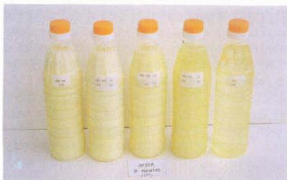
Figure 4(a). Cold stability of blends of single fractionated palm olein with sunflower seed oil after three months at 10°C. The blends are those listed in Table 1, with (L to R) 100%, 70%, 50%, 30% and 0% of palm olein.
