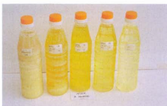
Figure 5(b). As Figure 5(a), but illustrating blends with double fractionated palm olein of IV65.
